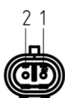
Diagram of black 2 Ways AMP terminal socket (temperature sensor)
